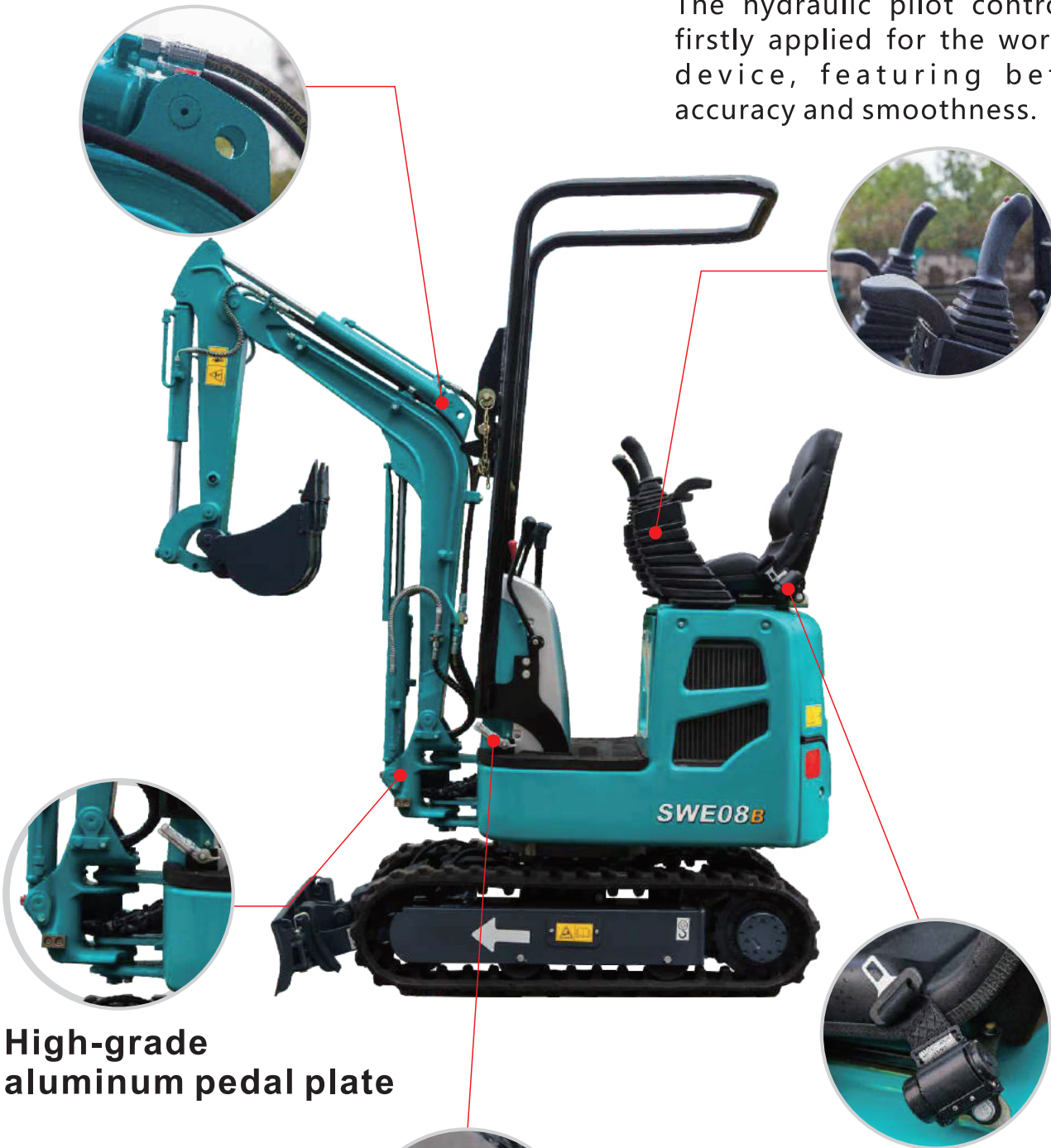
Concealed self-retracting seat belt
